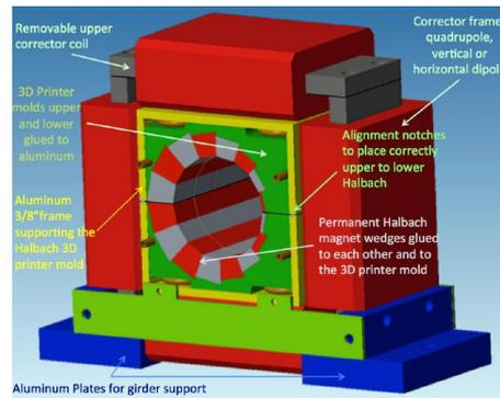
In 2017, a linear-field permanent magnet arc was tested at the Accelerator Test Facility (ATF-1) at BNL. It has a 6-cell approximately FODO lattice and bends through a total angle of 40 degrees. It transmitted beam through a kinetic energy range from 18 to 70.5MeV, demonstrating a ratio of 3.8x in momentum. Scans of the input beam position show transfer function from the beginning to the end of the arc are in line with predicted optics.
